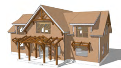
Timber Frame with SIPs & Exterior Elements
